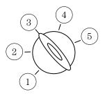
4. ON, all electrical circuits operational. Warning lights illuminated. Key position when driving.
